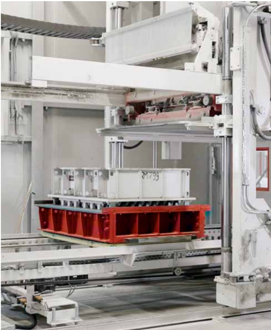
Hydraulic lifting system for quick mold change (optional)
