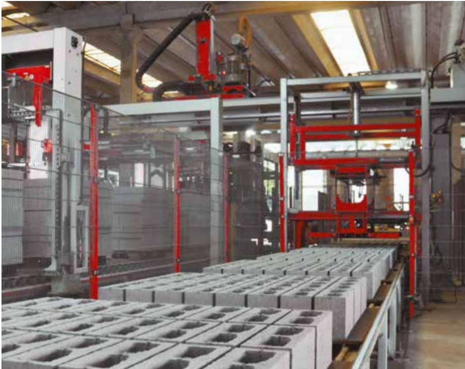
Dry side with hollow blocks
