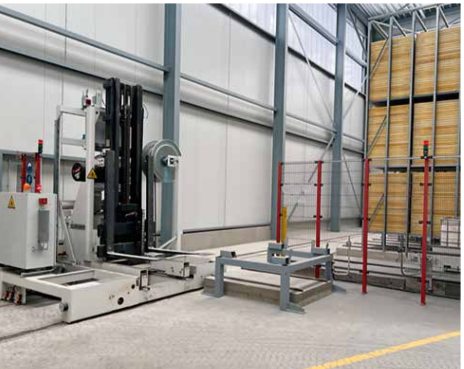
Finger cart system for board or steel pallet packages
