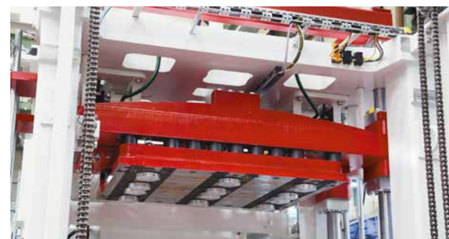
Rubberized tamper head plate (standard)
