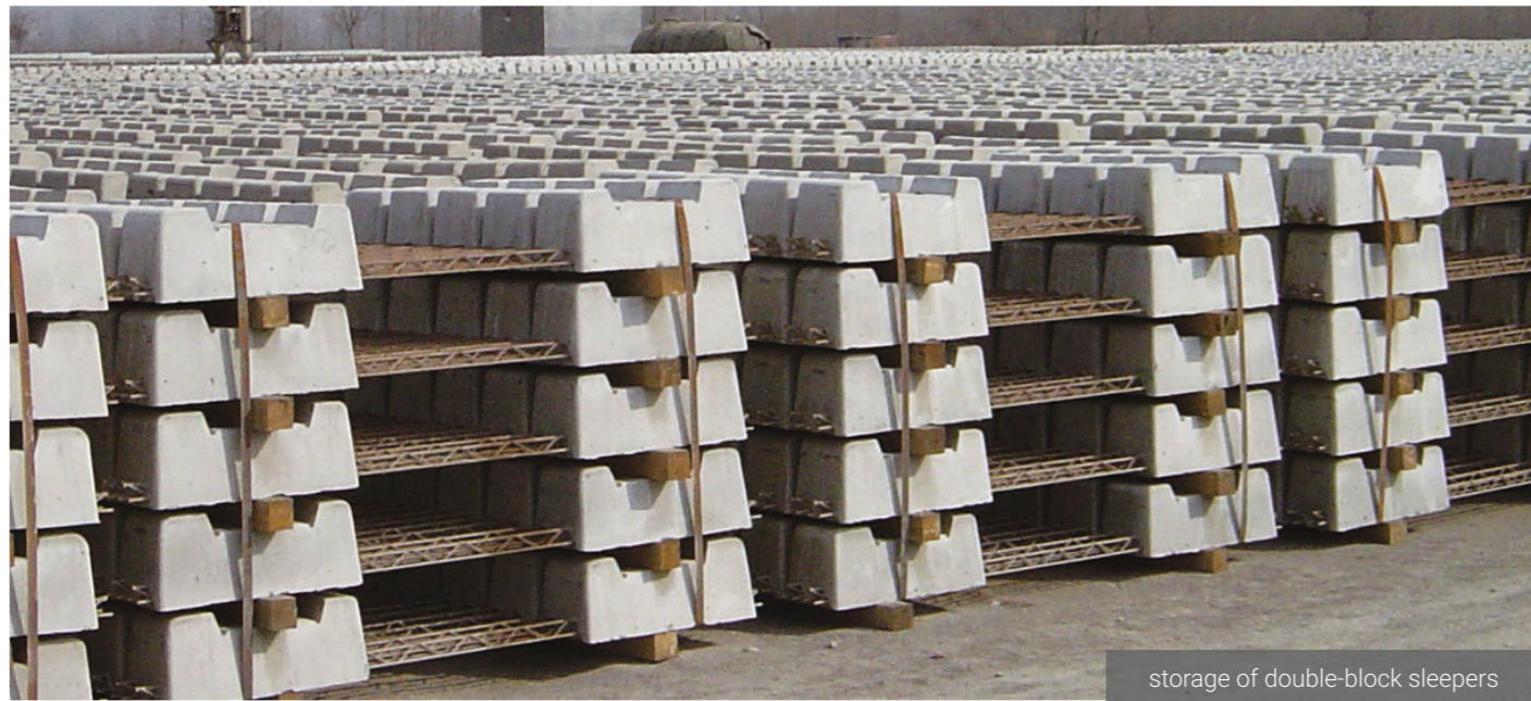
double-block sleepers with rail fastenings
