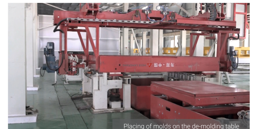
Mold handling device used for curing pit cover handling
